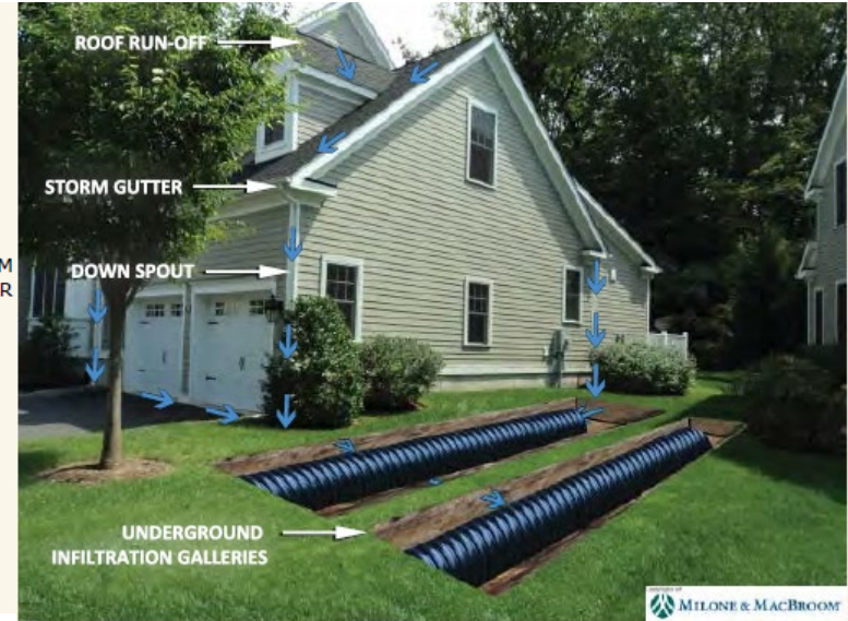
Typical infiltration gallery layout for residential properties
